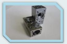
Hastelloy Valve MachiningApplication:Valves for mass flow limitersMaterial:HastelloyTolerance:±0.05 overall
